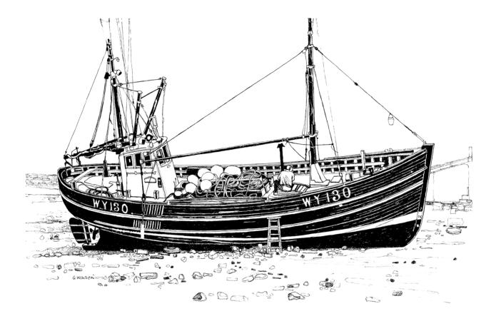
**11: OF SCOTTISH CONCEPT** — Whitby Boatbuilding produced some vessels of Scottish type. Designed with flydragging seining in mind, the 50ft *Accord* WY130 was delivered in 1958 to Skipper William Graham. She cost about £13,500 to construct.
